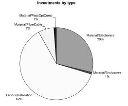
Fig. 5: Investments per type. The main costs are due to installations and electronics in FTTC
