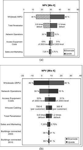
**Fig. 4:** Access equipment cost evolution is more highly critical for FTTO/H deployment (b) than for FTTC architectures (a). ARPU=Average Revenue Per User
