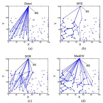
(c) (d) **Fig. 5.** Routing paths by Direct, MTE, SOR, and MaxEW with repeat events on the region from (0, 0) to (50, 50).
