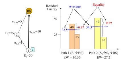
Fig. 1. An explanatory example for Energy Welfare Routing algorithm: Node 1 routes data to a path to maximize an Energy Welfare (Average×Equality) of sensor 1 and 2.
