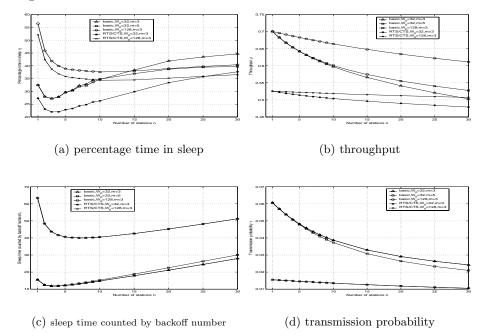
Fig. 2. The performance of the 802.11 network executing the sleep algorithm.
