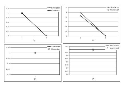
Fig. 5. Probability distribution of the number of bursts. IPP arrivals, no residual,  $B_{min} = 0$  bytes, Average Arrival Rate = 1 Gbps
