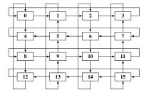
Fig. 2. 4×4 Manhattan street-based simulation network
