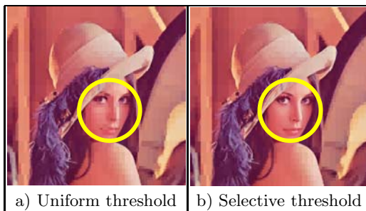
Fig. 3. Lena Image with Selective Threshold Regions. It can be seen that with selective threshold to preserve the facial details, the lena image is visually higher quality than the same image with uniform threshold across the image
