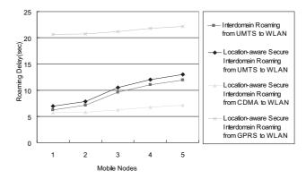
Fig. 7. Delay performance of Location-aware Secure Roaming from 3G to WLAN
