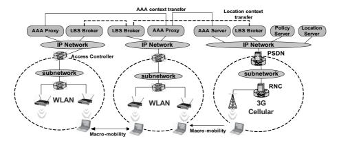
$\textbf{Fig. 5.} \ \, \textbf{Testbed} \ \, \textbf{of the Location-aware Security Architecture for UMTS/WLAN interworking}$
