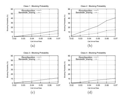
**Fig. 2.** Blocking probabilities of new and handoff calls (a) class 1 (conversational) (b) class 2 (streaming) (c) class 3 (interactive) (d) class 4 (background)
