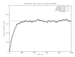
**Figure 6:** Dynamic tracking of gTrace over a full 8-ary tree of height 3 with 512 potential receivers.
