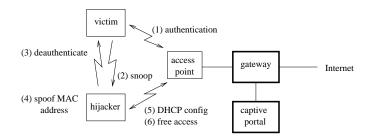
Fig. 2. Low-level 802.11 vulnerabilities allow a hijacker to gain control of a session of an authorized user.
