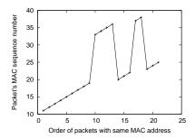
Fig. 4. Freeloading causes interleaving of different senders' MAC sequence number trend lines
