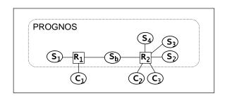
Figure 7: The topology of the Prognosfs testbed. An  $S_x$  is a Stone. A  $C_x$  is a "client". An  $R_x$  is a network switch that houses no disk and is not programmable.  $R_1$  is a Netgear Fast Ethernet Switch FS108.  $R_2$  is an Intel Express 510T Switch. All links are 100 Mbps.
