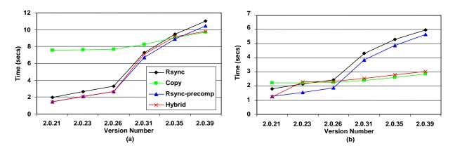
Figure 3: Performance of pair-wise exchange. (a) The link bandwidth is 25 Mbps. (b) The link bandwidth is 100 Mbps.
