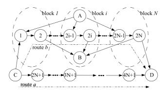
**Fig. 1.** Sample graph topology. All link capacities and weights equal to 1 and there are N and 1 units of demand for  $A \to B$  and  $C \to D$ , respectively
