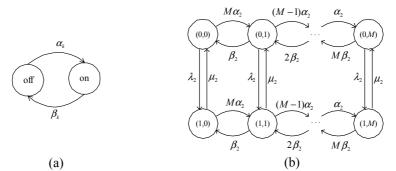
**Fig. 1.** Traffic Models with (a) a 2-state Markov chain for an on/off source and (b) a 2-dimensional Markov chain for a video source
