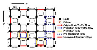
**Fig. 1.** Concatenated rings on mesh(6,6) for path protections.
