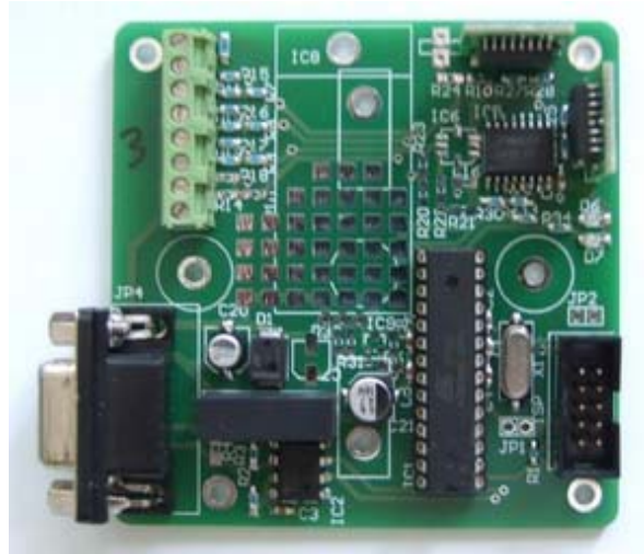
Fig.6. The sensors' controller board.
