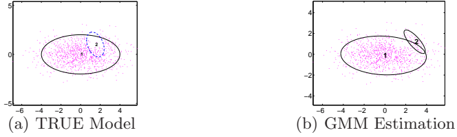
Fig. 1. Samples generated by a component and partly absorbed by another one (average log likelihood in (a) and (b) is 0.353 and 0.351, respectively ).
