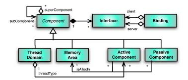
Fig. 2. A Real-Time Component Metamodel
