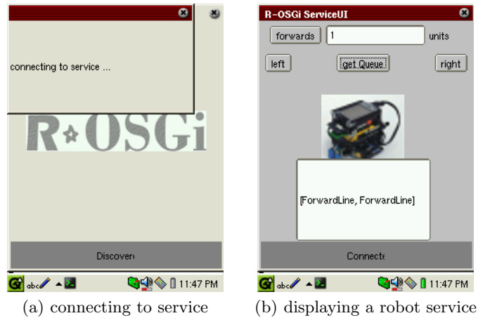
Fig. 4. ServiceUI for an R-OSGi-driven Lego Mindstorms Robot on a Zaurus PDA
