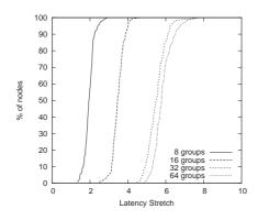
Fig. 3. Latency stretch for 128 subscriber nodes, when varying the number of groups.
