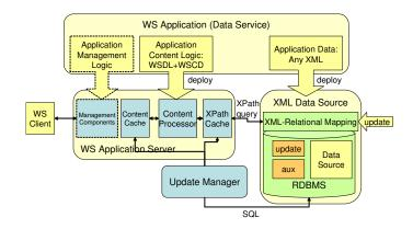
Fig. 1. WReX: Web Service Caching Architecture
