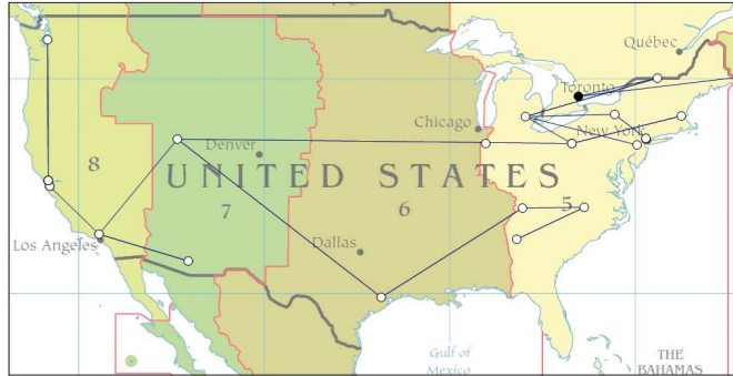
Fig. 6. The real-time wide-area topology produced by the node stress aware algorithm after 30 nodes have joined (only nodes that reside in North America have been shown, some nodes may reside in the same geographical location).
