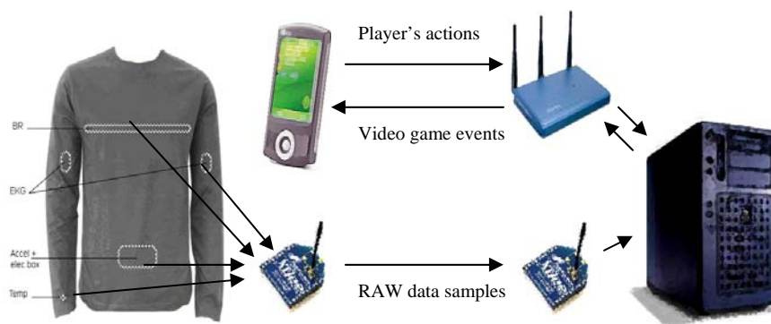
Fig. 1 Position of the various sensors on the tee-shirt, wireless Zigbee and Wifi networks.
