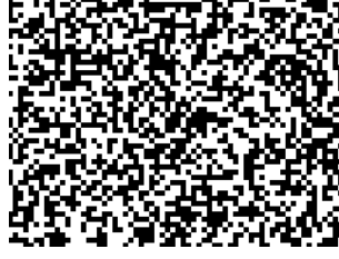
Fig. 4. A part of 2-D binary De Bruijn sequence with 64 \times 48 resolution. The pattern is enlarged to make every code bit distinguishable to the reader. Note that there is no repeated 5 \times 5 sub-window in this pattern.
