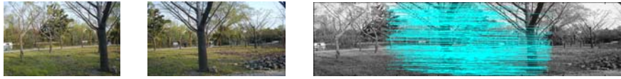
Figure 3: Original images (the left two images) and SIFT feature matches extracted from a pair of images (right)
