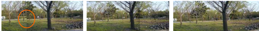
Figure4: the image after stitching using the method based on area [2] (the matching error is marked with red rectangle) and using the method based on SIFT features with obvious seam (middle) stitching result after smoothing the transition (right)
