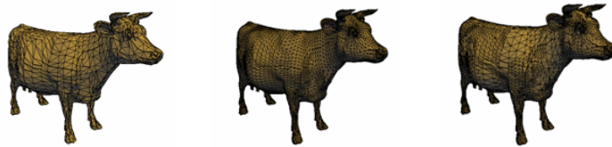
Fig. 4. The PM of cow: the left model with 4000 triangles is initial control mesh, the middle one with 16000 triangles is the result after performing one step global Loop subdivision, the right one is the result after performing one step adaptive subdivision with sharp features.
