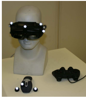
Fig. 7. The head mounted display and props used in the prototype system: upper left is an optical see-through HMD equipped with stereo circular-polarizing filters in its front, lower is a prop with buttons held by the hunter, and on the right is a game pad used by the driver. A set of infrared reflective markers were attached to the devices needed for tracking.
