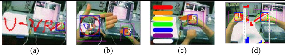
Fig. 2. (a) Memo by using a virtual pen (b) a saved image is augmented on the palm. (c) Change color of a pen (d) the user can move blocks using the finger tips in the Tetris game
