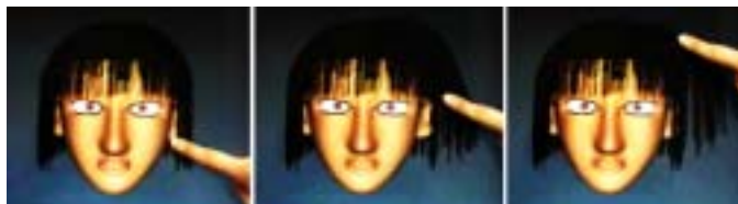
Fig. 10.2. Changes when the robot's hair is stroked from the ends to the roots
