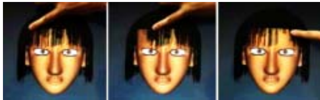
Fig. 9.1. Changes when the robot's fringe of hair is stroked from left to right
