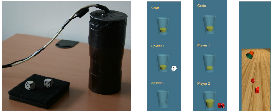
Fig. 3. The CamCup (left) and different GUI states (right). The cup is augmented by a webcam which registers the casts. Basically, three GUI states can be distinguished: (i) Rating announcements (left), (ii) casting dice by user (middle), (iii) casting dice by agent (right).
