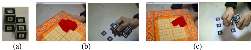
Figure 2. Pueblo interface (a) Shape of the interface (b) Visible markers at varying positions (c) Two-hand interaction
