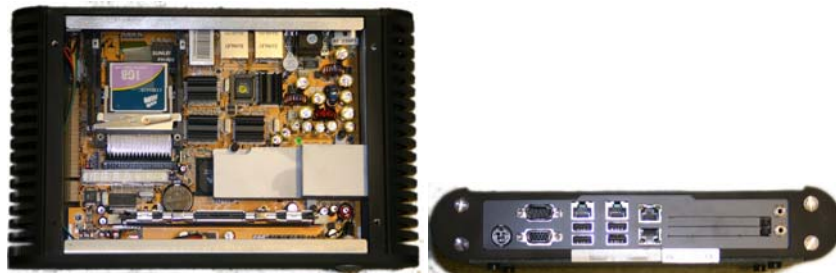
Fig. 1. Internal and connections views of the industrial autonomic network node.
