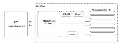
Fig. 1. Testbed–PC and IXP1200 router
