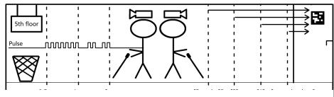
Figure 2. Vibrotactile cues and navigation instructions depend on the distance to the obstacle (left side) or marker (right side).
