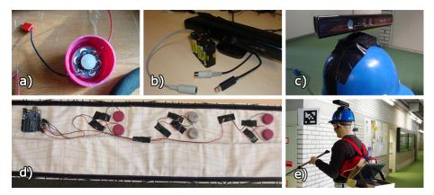
Figure 1: (a) LilyPad vibe board in a plastic cap. (b) Mobile Kinect camera with battery pack. (c) Kinect helmet. (d) Vibrotactile Waist Belt. (e) Complete setup with backpack.
