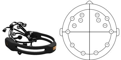
Fig. 1. A low-cost EEG device (Eomtiv EPOC neuroheadset [10]) and layout of EEG channels.
