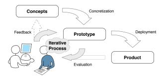
Fig. 1: Overview of the User-centered Design procedure.
