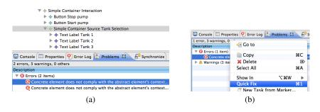
Fig. 11: Problems View of the Eclipse tool: The validator has recognized semantical incorrectness between the CAP3 model and the altered Movisa model (a) and provides means to fix it (b).
