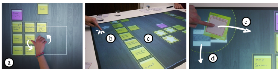
Fig. 4. Focusing on a specific region in the workspace (a); searching for notes (b,c); retrieving and adding images based on the content of notes (d,e).
