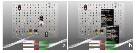
**Fig. 5.** (a) Participants share a synchronized logical view from different PCs and are able to simultaneously enter search criteria into the text boxes; (b) Via the slider widgets that are assigned to the text boxes, it is possible to adjust the weight of search criteria.
