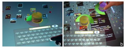
**Fig. 4.** (a) A Search Token as hybrid surface on a multi-touch tabletop display enable users to simultaneously enter search criteria via on-screen keyboards; (b) By turning a Search Token, the weight of a search criterion can be adjusted.
