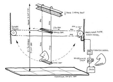
Figure 2 Illustration of mechanism of rope swing
