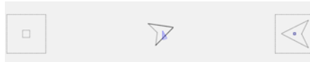
Fig. 4. The experimental task consisted of docking a triangular shaped object over a target. Rotation is controlled using pressure, and displacement controlled with mouse movement.
