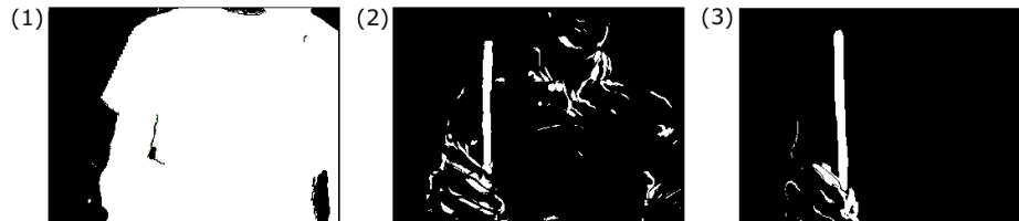
Fig. 4. Analysis of movement with difference-images, (1) With background as reference-image, (2) With three following images, movement of the body, (3) With three following images, only movement of the arm
