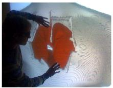
Figure 5: Two examples of applications interfaced by the iMUTS interaction paradigms. (Left) a user interacts in a landscape-planning scenario on an FTIR multi-touch wall with an anaglyph-based stereoscopic projection. (Right) a user performs volume deformation in a medical scenario using a large FTIR-based passive back projection iMUTS.
