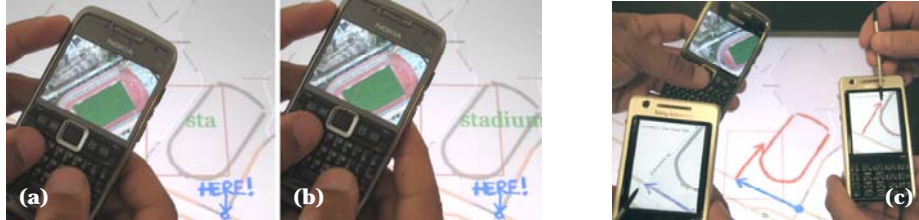
Fig.2. a–b) The lack of tactile buttons on the surface can be addressed by using the physical keyboard of the mobile device. Here, the user enters “Stadium” on a point of interest. c) Simultaneous input from multiple uniquely identified devices allows collaborative scenarios. A blue arrow has been drawn on the left device, while a red arrow and an outline of the stadium has been added using the right device.
