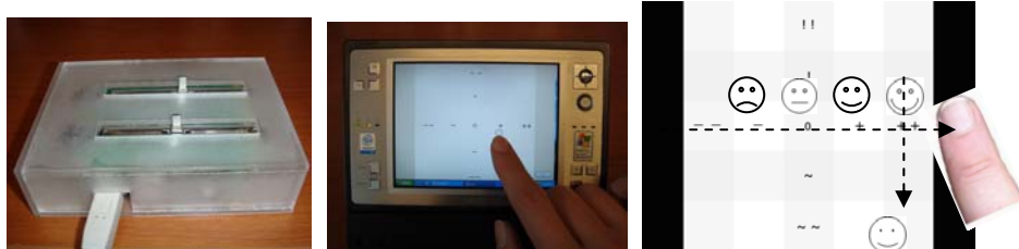
Fig. 1a. Two-slider Emotrace; 1b. Touchscreen Emotrace; 1c. Dynamic Facial Feedback: The mouth changes with horizontal motion; the eyes change size with vertical motion.
