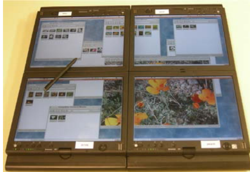
Fig. 1. Four individual tablet computers, linked only by a wireless network, forming a multi-display composition resulting in a single logical display.
