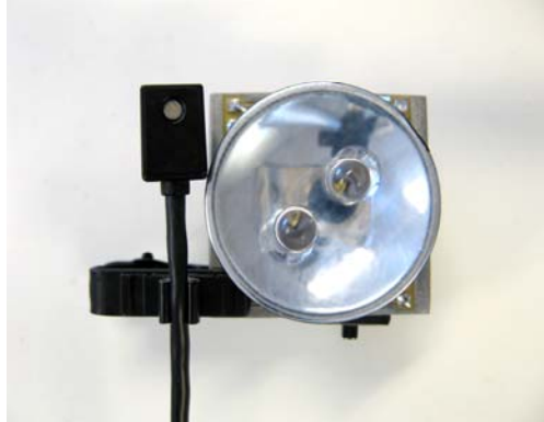
Fig. 2. Lapel mike with wireless infrared tag.
