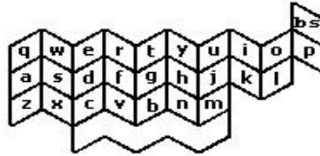
Fig. 3. The accordion virtual keyboard with 120° of folding angle.
