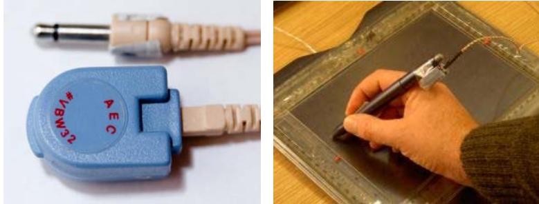
Fig. 2. Tactaid VBW32 transducer (left). Tactaid mounted on the pen of the tablet (right)
