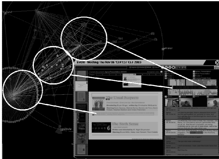
Fig. 9. In the integrated meeting browser, media can be synchronously played, thanks to the temporal alignments. Further, since topics evolve during a meeting, links and relations to the documents in the whole meetings archive dynamically change over time.
