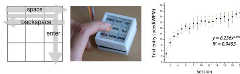
Fig. 2. Implementation and evaluation of Button Keyboard (left: finger gesture as commands, center: prototype, right: text entry speed of Button Keyboard)
