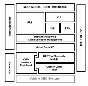
Fig. 2. System architecture.
