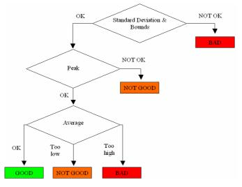
Fig. 6. Oxygen Test evaluation flow chart.
